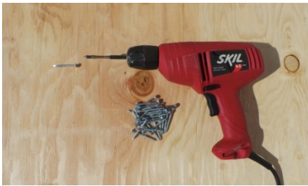
Power drill & 2" woodscrews (28 ea.)
