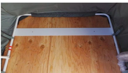
Use the same 1.5: bolts, nuts, and washers to secure the anchor plate (2 holes).
